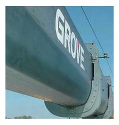
The Grove MEGAFORM<sup>™</sup> boom shape eliminates weight and increases capacity compared to conventional shapes.
